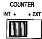
Selects internal or external counter function. To view an external signal's frequency, the Function Counter must be in the EXT position.
