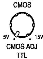
This knob becomes effective when the TTL/CMOS output is connected (page28).
