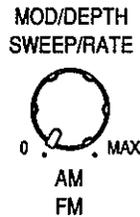
The Sweep Rate knob sets the frequency width. The current output frequency becomes the start frequency.
