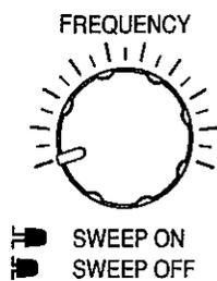
3. Use the frequency dial to adjust the frequency of the GCV output.
