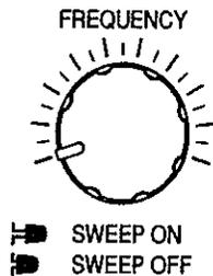
3. Use the frequency knob to set the frequency. For best results set the frequency knob to its most clock-wise position, this will set the upper frequency limit.
