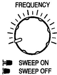
3. Use the frequency knob to set the frequency. This will set the upper frequency limit.
